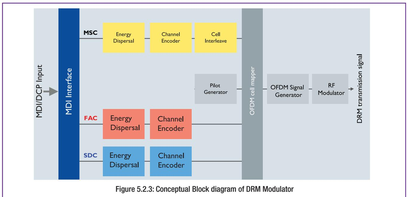
Figure 5.2.3: Conceptual Block diagram of DRM Modulator
