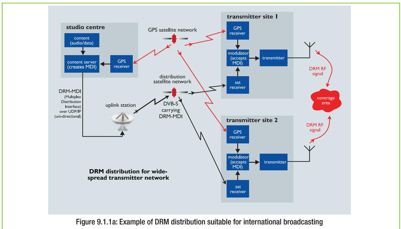
Figure 9.1.1a: Example of DRM distribution suitable for international broadcasting
