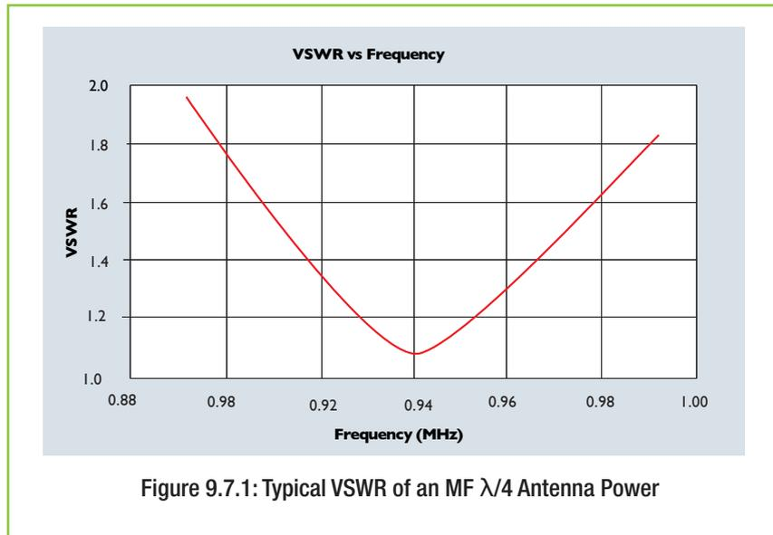
To illustrate this, the basic Voltage Standing Wave Ratio (VSWR) characteristic for typical single  $\lambda/4$  resonant mast radiator is shown in Figure 9.7.1. This characteristic refers to a base fed 75 metre mast, having a diameter of 0.5 metre, and was obtained by NEC modelling. The resonant frequency is approximately 939 kHz.
