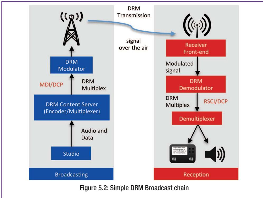
In the following sections we will examine the operation of the two main functional blocks shown above: the Content Server and the Modulator. In most (but not all) installations, these functional blocks correspond to commercially available products. They communicate via a Multiplex Distribution interface (MDI) over a Distribution and Communications protocol (DCP), both of which have been standardised [2], [3].
