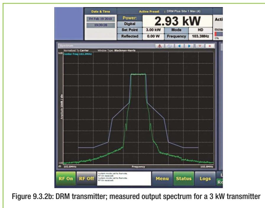
Figure 9.3.2b: DRM transmitter; measured output spectrum for a 3 kW transmitter
