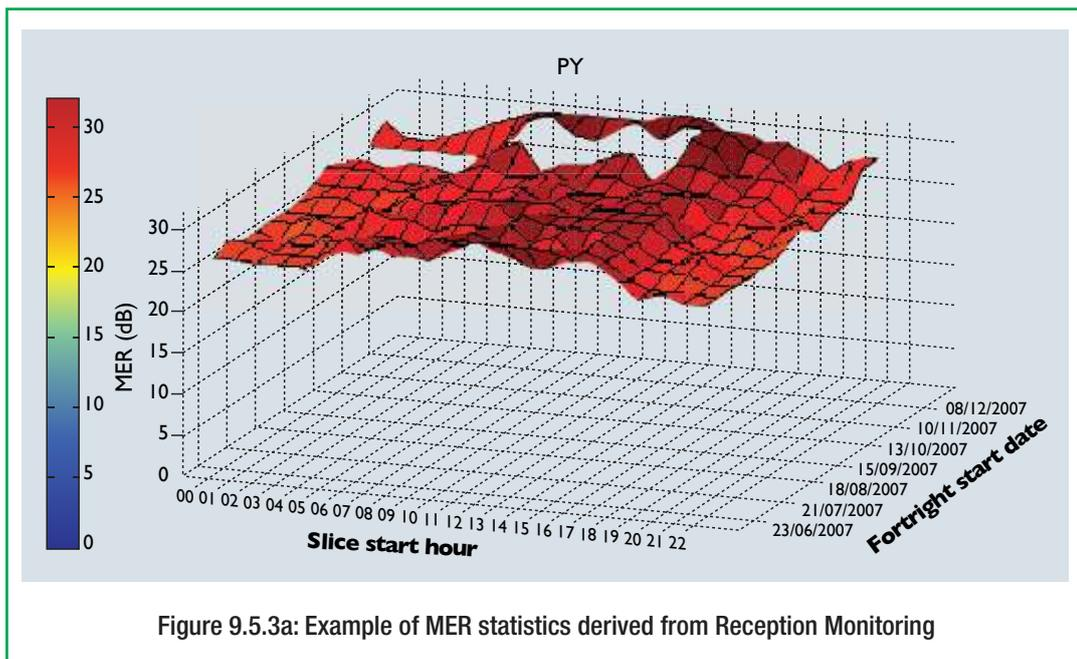
Figure 9.5.3a: Example of MER statistics derived from Reception Monitoring
