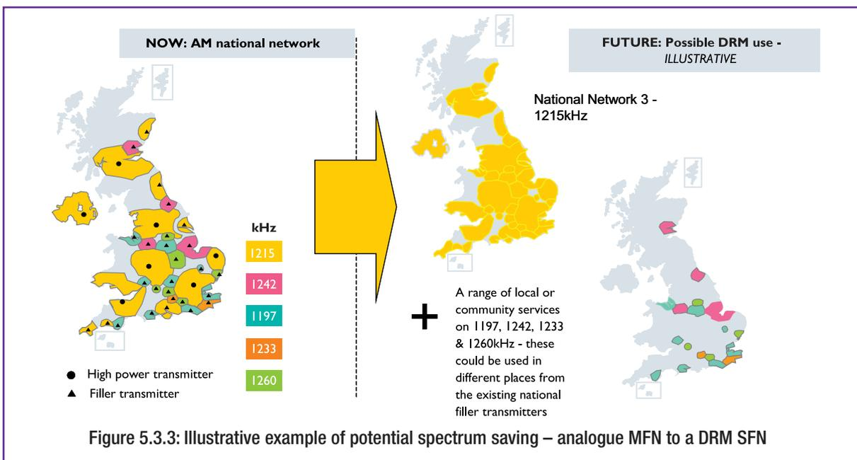
Figure 5.3.3: Illustrative example of potential spectrum saving – analogue MFN to a DRM SFN
