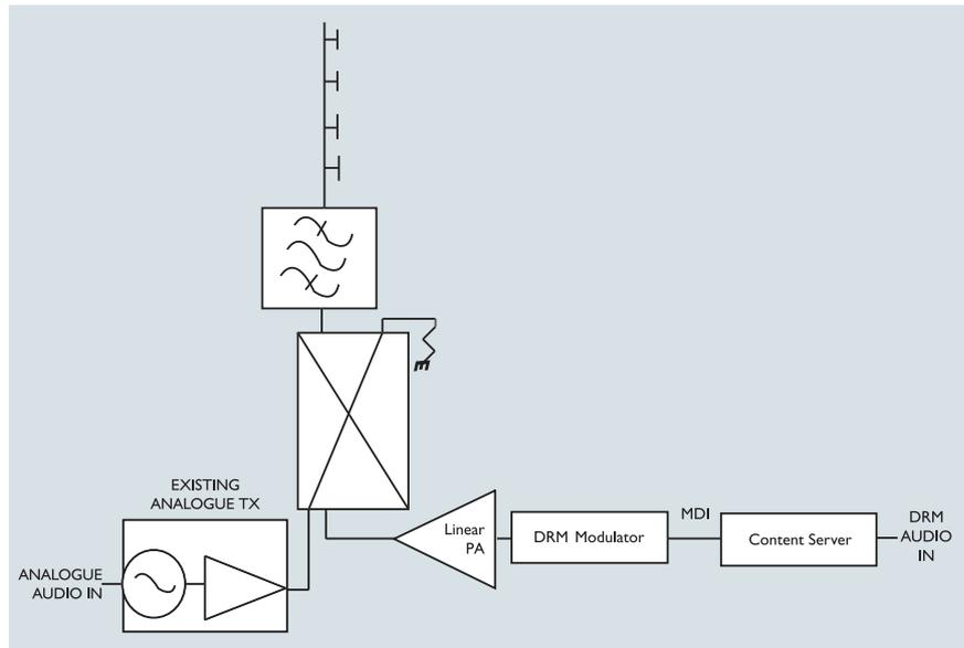
Figure 9.3.3.1: DRM combined mode with RF power combining
