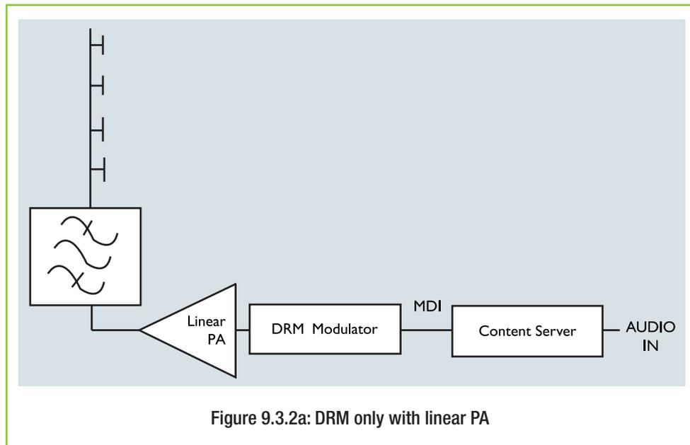
Figure 9.3.2a: DRM only with linear PA
