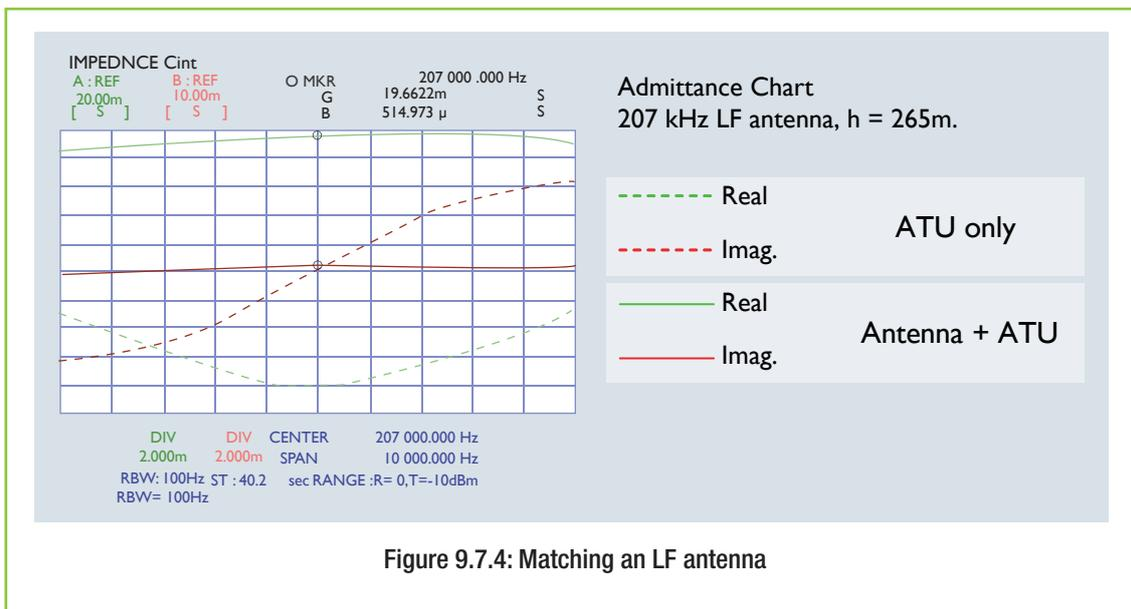
Figure 9.7.4: Matching an LF antenna
