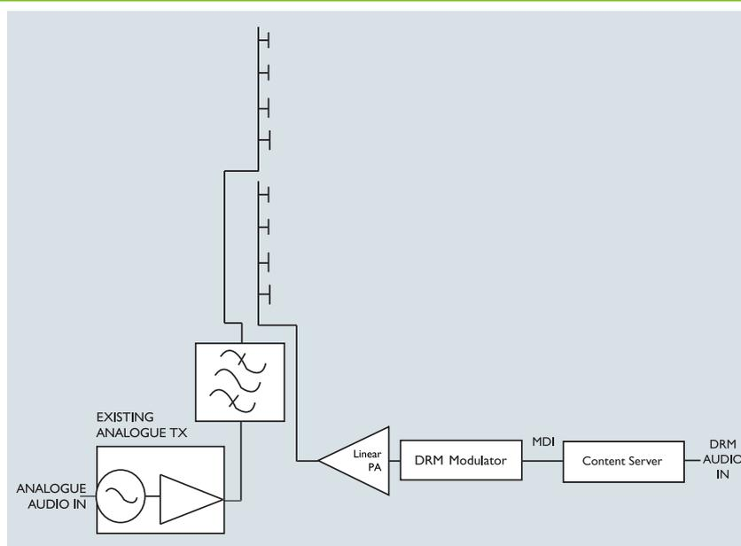
Figure 9.3.3.2a: DRM combined mode antenna coupling
