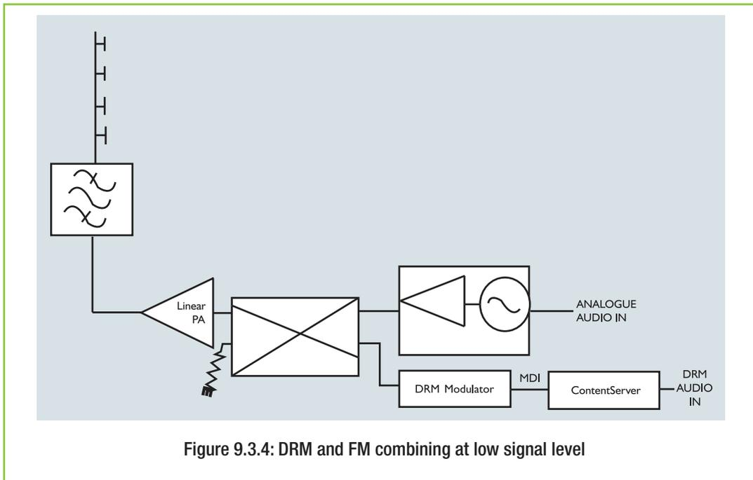
In this configuration the DRM signal and the FM signal are combined in front of the power amplifier. The coupling is done at low signal level and the energy losses on the dummy load resistor connected to the hybrid coupler is insignificant.
