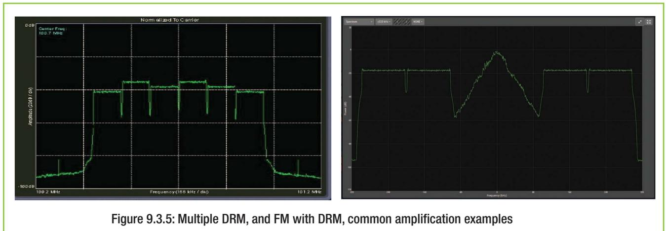
Figure 9.3.5: Multiple DRM, and FM with DRM, common amplification examples
