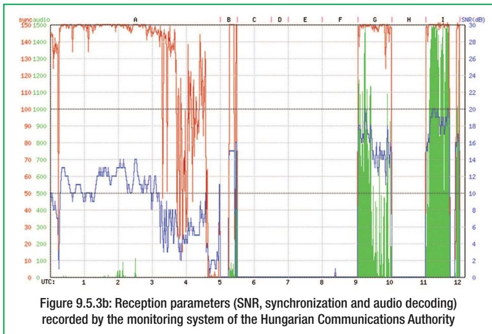
Figure 9.5.3b: Reception parameters (SNR, synchronization and audio decoding) recorded by the monitoring system of the Hungarian Communications Authority
