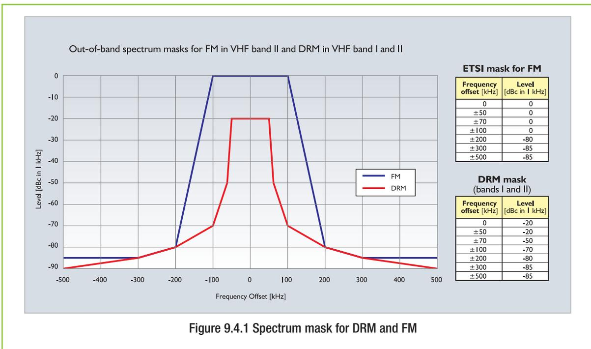
Figure 9.4.1 Spectrum mask for DRM and FM
