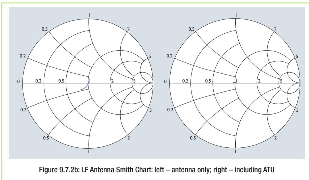
Figure 9.7.2b: LF Antenna Smith Chart: left – antenna only; right – including ATU
