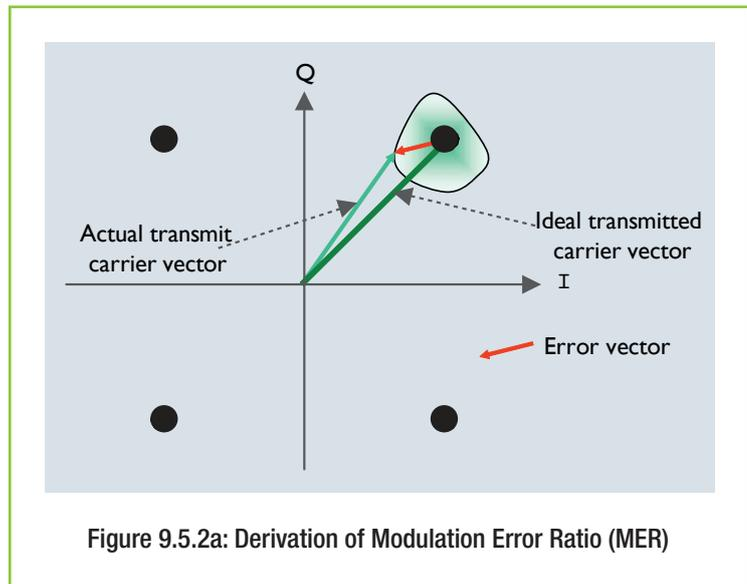
Figure 9.5.2a: Derivation of Modulation Error Ratio (MER)
